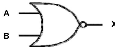
This is basically an **OR** gate with the output X inverted.
