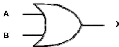
The output (called X) is **true** (i.e. **1** or **ON**) if the (**INPUT A OR INPUT B**) are **true** (i.e. **1** or **ON**).
